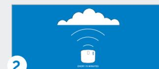
The data collected from the sensor is delivered real-time (via 3G) to the cloud (every 15 minutes).
